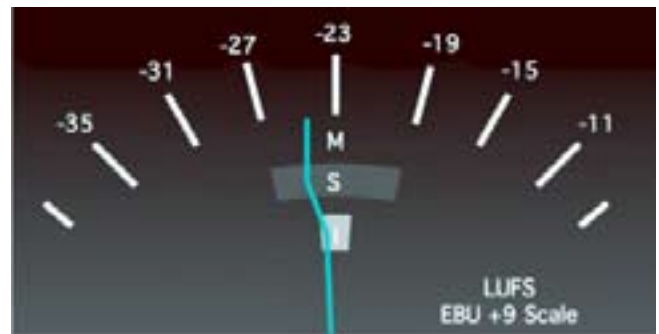
Figure 7: A schematic representation of an emulated loudness meter with a “bendy needle”
